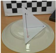
The scene will consist of a central frame. It is defined as being right handed with the *x-axis* defined as being oriented towards the camera (parallel to the table surface) and the the *z-axis* upwards (presumably in line with the gravity normal) and the *y-axis* being orthogonal to these axes (see illustration at left)
