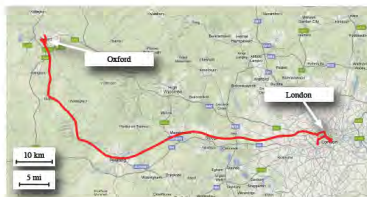
Figure 1: 121 km path between Oxford in the upper left and London in the bottom right. We compute visual estimates for 89.4% of this distance. Using appearance-based place recognition and inertial dead reckoning, 100% is covered topologically, which is sufficient for path planning. The graph begins in an office in Oxford, and proceeds with various forms of transport including: foot, bicycle, train, subway, escalator, rickshaw, punting-boat and ferris wheel. Note that we cannot detect our true position in the global inertial frame – when we are traveling on the train or subway for instance, motion with respect to the global inertial frame becomes effectively unobservable in the presence of noise.
