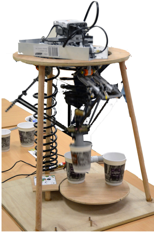
Fig. 1. The Delta Cup Robot was designed as part of an autonomous cup arranging and filling project where cup and condiment locations are not known in advance. This involves several principles including object recognition, kinematics/control, and motion planning and compliance
