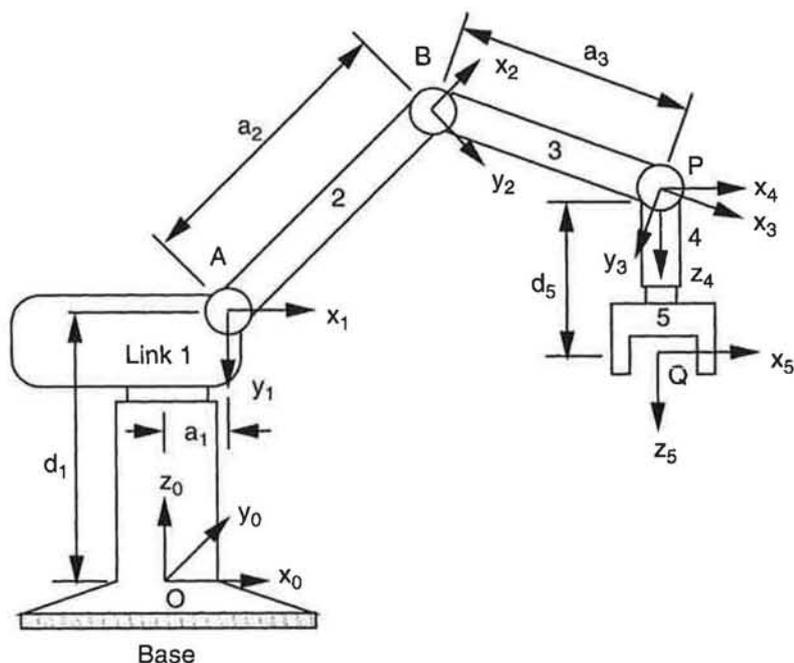
FIGURE 2.5. Schematic diagram of the Scorbot robot.
