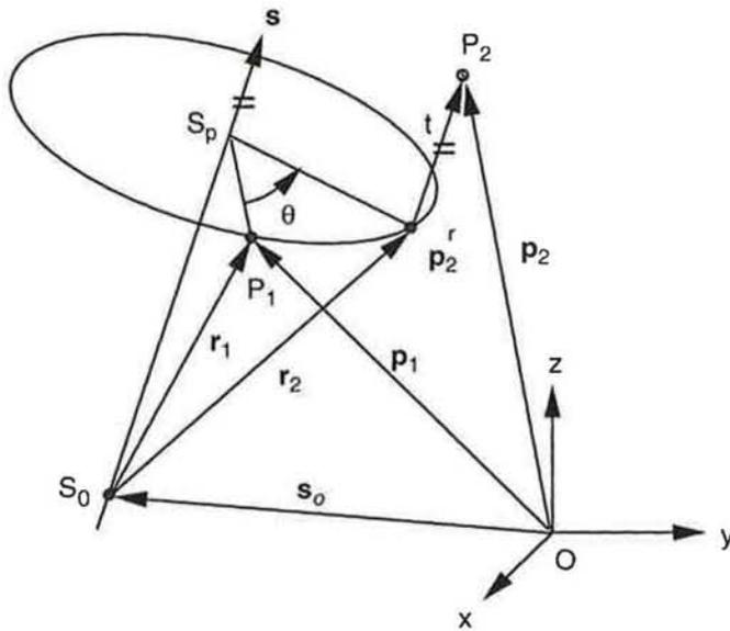
FIGURE 2.12. Vector diagram of a spatial displacement.
