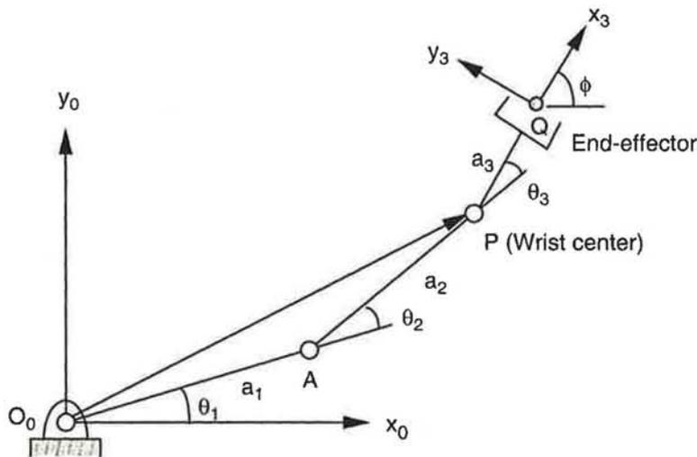
FIGURE 2.7. Vector loop of the planar 3-dof manipulator.
