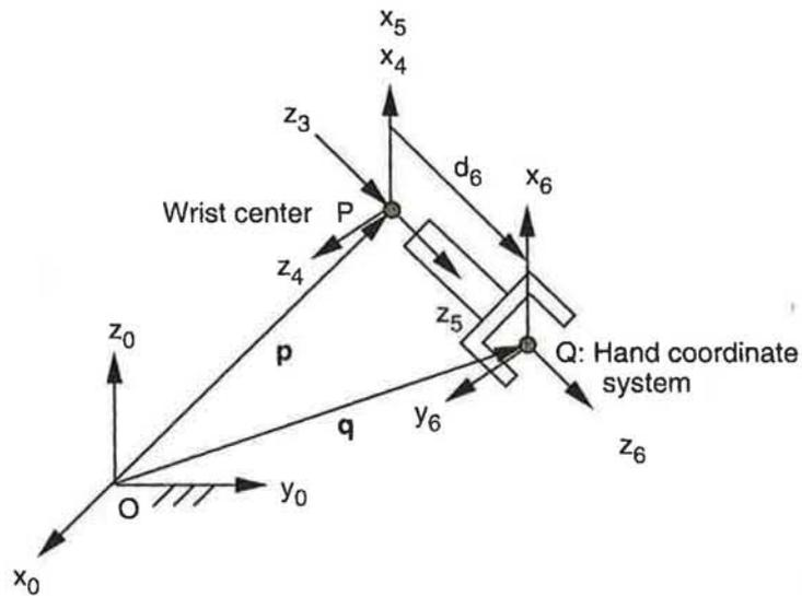
FIGURE 2.9. Hand coordinate system and wrist center position.
