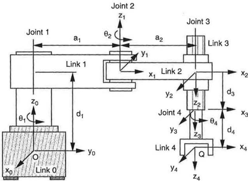
FIGURE 2.4. Schematic diagram of a SCARA arm.
