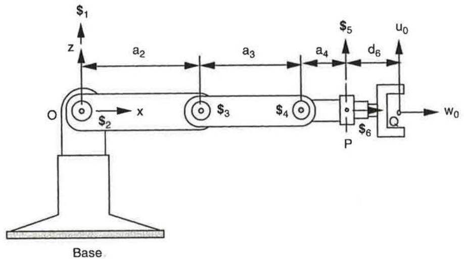
FIGURE 2.16. Reference position of the elbow manipulator.
