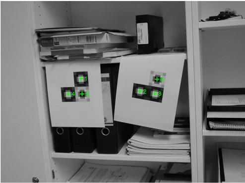
Figure 13: Two out of eight possible 3-bit marker arrays photographed with a Sony DSC-S85 at resolution 2272×1704 pixels. The location of the six SURF features which yielded highest detector response are displayed as green crosses.
