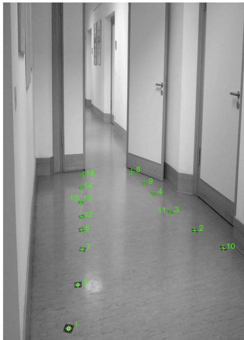
Figure 10: Image captured with a Panasonic DMC-FX1 at resolution  $2048 \times 1536$  pixels, after vertical upsampling by factor 2. The detected SURF markers are labelled according to the ranking in Figure 11.
