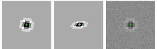
Figure 6: Examples of the distortions we applied to the SURF marker in our synthetic experiments. In plane rotation by  $10^\circ$ , out-of-plane rotation by  $40^\circ$ , Gaussian noise with standard deviation equal to 50 gray values. The green cross indicates the position at which the marker has been detected
