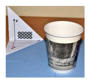
**Base:** The coordinate frame we wish to work in is cartesian and is located *at a base/corner origin of the Workspace*. The origin of the workspace is indicated by a right-handed <u>UQ Robotics frame</u> with a tag. It is oriented with the *z-axis* orthogonal and upward to the gravity-normalized horizontal plane with the *x-axis* defined as being along a scene relative edge (see illustration at left).
