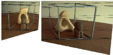
(b) Image pair transformed by the specialized projective mapping  $H_1$  and  $H'_1$ . Note that the epipolar lines are now parallel to each other in each image.
