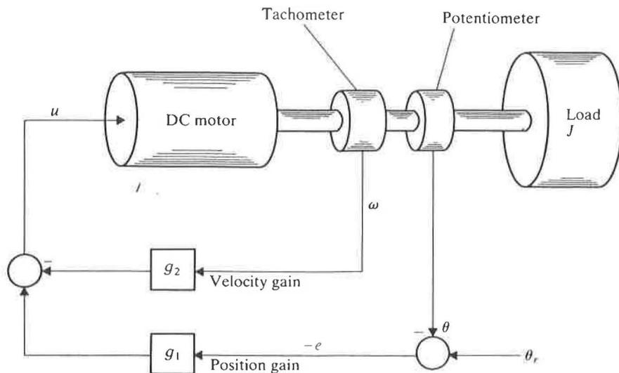
Figure 6.2 Implementation of an instrument servo.
